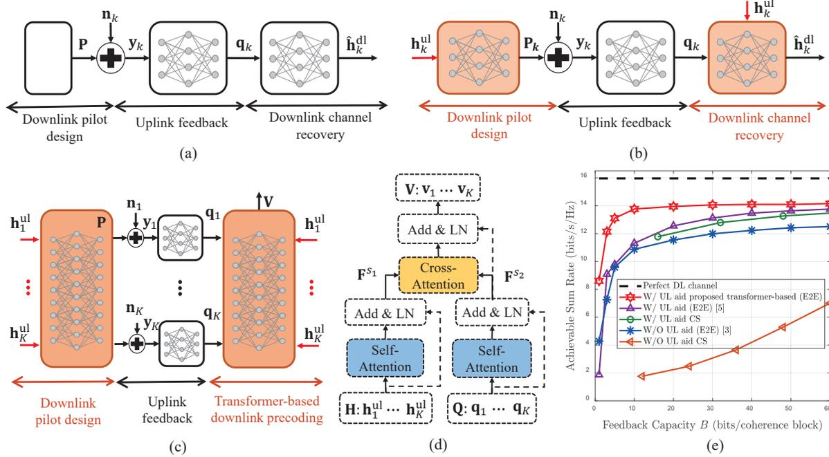
**Figure 1** (a) The E2E scheme for downlink channel estimation without uplink aid [3], (b) the E2E scheme for downlink channel estimation with uplink aid [5], (c) the proposed transformer-based E2E scheme for downlink precoding with uplink aid, (d) the proposed transformer-based precoding model, and (e) the comparison of achievable sum rate performance.
